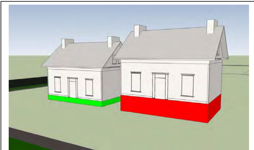
Oversized foundations are out of context with the Village of Bath (shown in red). A more modestly sized foundation (shown in green) is more contextually appropriate with heritage structures.
