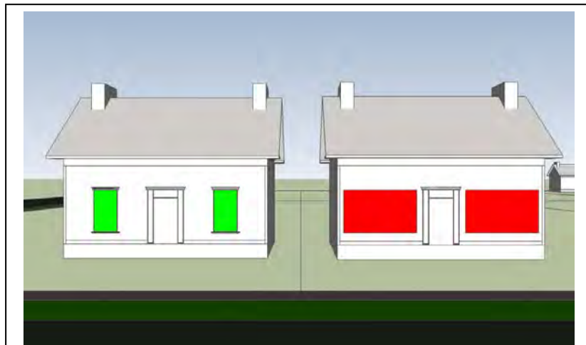
The proportion of solids and voids is significant to the reading of a structure. The building on the left (shown in green) has appropriately sized windows in relation to the wall space and door. The building on the right (shown in red) has oversized windows that dwarf the door and overwhelm the building's façade.
