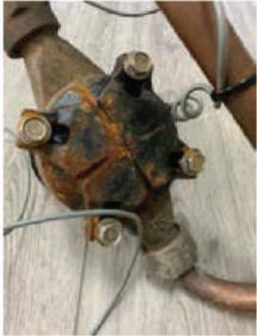
This picture shows the underside of a water meter removed from a building that was unheated during the winter months. The frost plate of the meter is cracked from the water in the meter having frozen and expanded.
