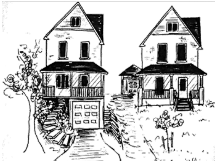
Images 3 & 4: Two examples of garage additions to a heritage building. One has been added below the building's façade and the other is detached and placed behind the structure. Both examples are in keeping with the scale and massing of the original buildings as they are subordinate to the houses and designed for one car (Amanda Sherrington, 2013).
